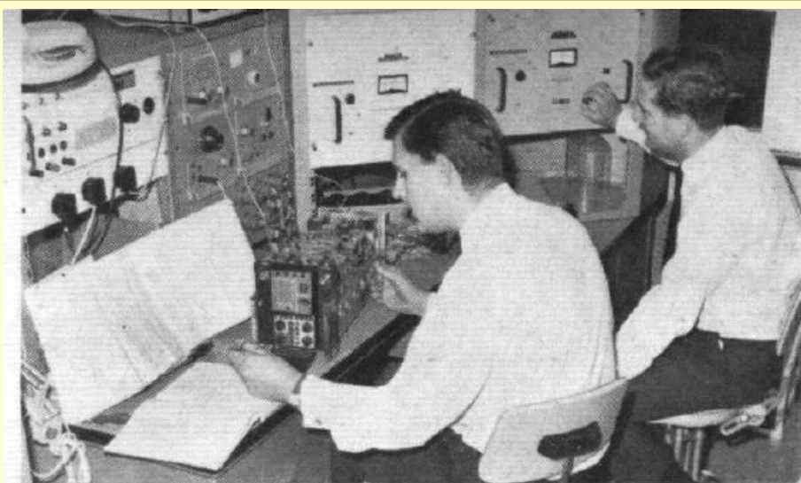
Final check being made on the first of the Elliott modular air data computers for the USAF C-5A Galaxy. This unit is the first of an order running to well over a hundred computers ordered by Lockheed last September
