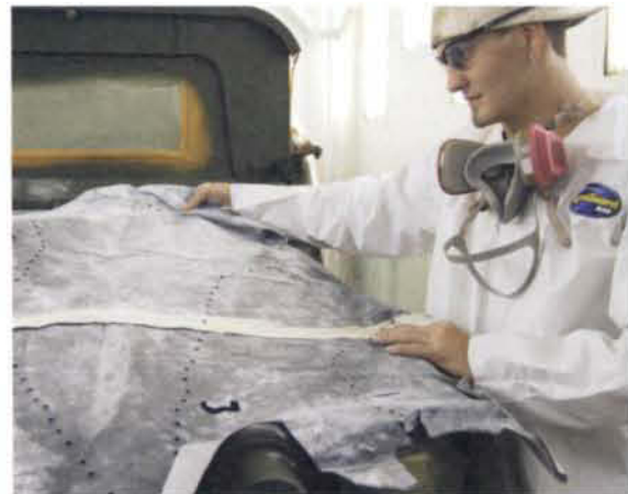
Above: Josh Sawyer applying a stencil to guide the CAMO painting, and left, a completed CAMO painting of the M1114 HMMWV
