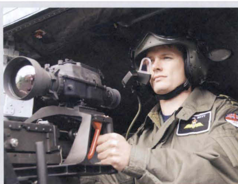
Above: the remote sighting system will give door gunners on Lynx helicopters greater capabilities
