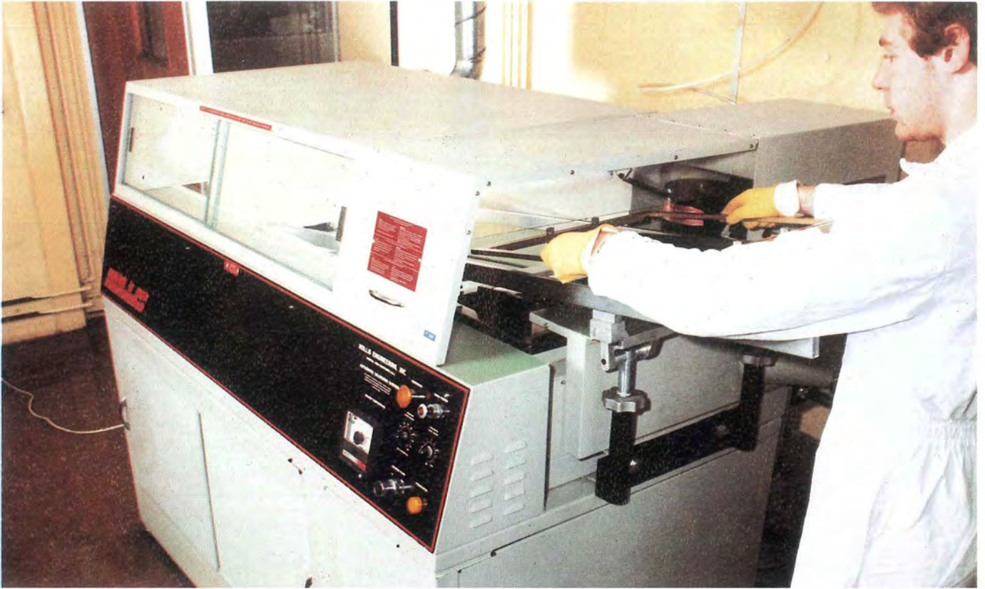
Wave Soldering Facility
