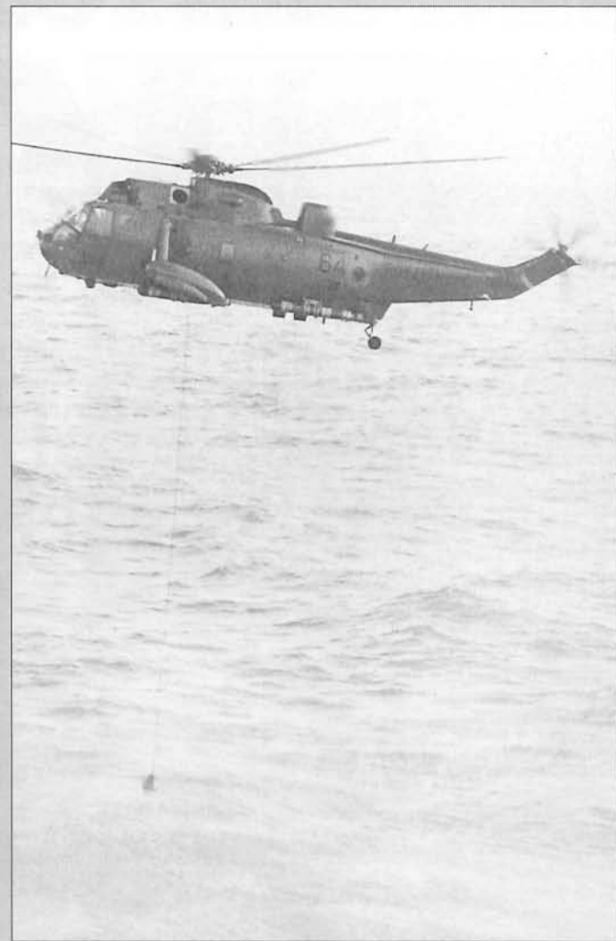
A hovering Sea King dips the sonar equipment into the sea.
