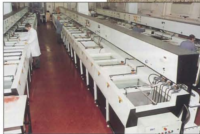
The newly constructed Material Process Plant at Rochester has been specially built to provide the Group with a facility enabling the surface of metals to be plated to a very high standard. Many highly toxic and corrosive substances are used to obtain the appropriate finish, all are controlled in both storage and usage to a high degree of safety. The Plant itself satisfies the Southern Water Authority that the trade effluent discharged is well within the stringent limits set by that Authority.
