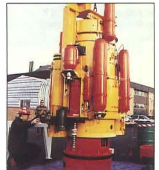
Gary Wallington, Senior Production Engineer, checks alignment of Subsea Control Module and Installation Tool during testing at GEC-Marconi's Nailsea facility.
