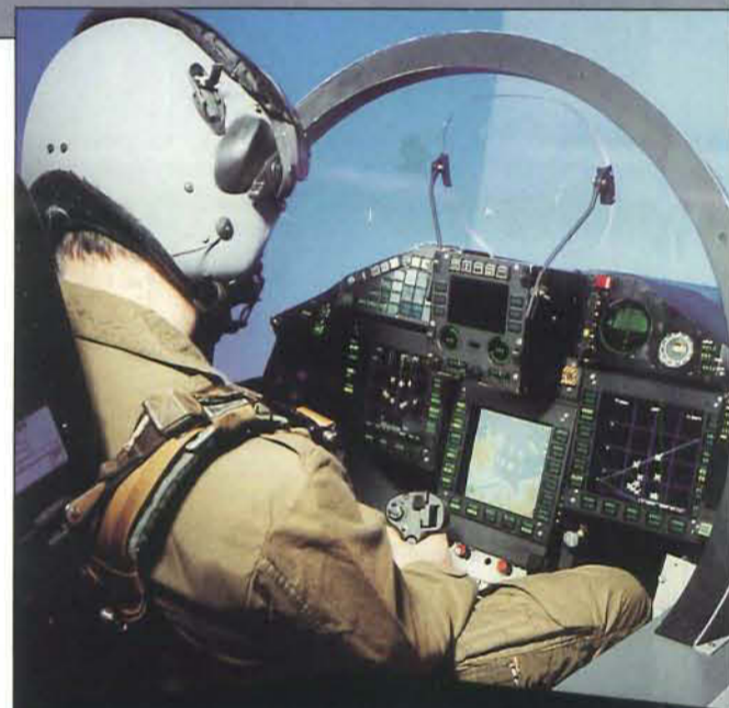
The EF2000 cockpit, designed to deliver optimum levels of tactical and functional information to the pilot without overloading him. The HUD is clearly visible at the centre of the picture.
