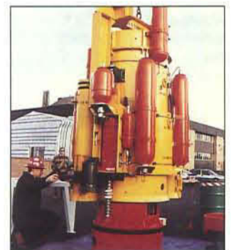
Gary Wallington, Senior Production Engineer, checks alignment of Subsea Control Module and Installation Tool during testing at GEC-Marconi's Nailsea facility.
