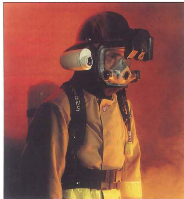
Fireman's helmet - one in a range of infra-red thermal imaging equipment that operates without special cooling.
