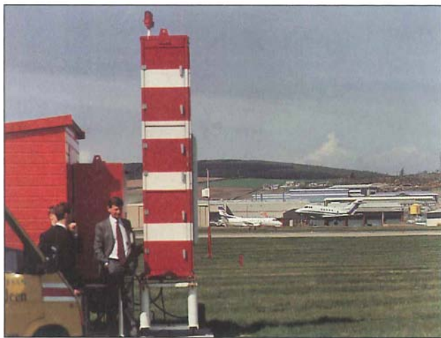
The Company jet about to touch down at Aberdeen at the end of a demonstration of the tri-mode ILS/MLS/GPS equipment. The MLS ground installation is on the left.
