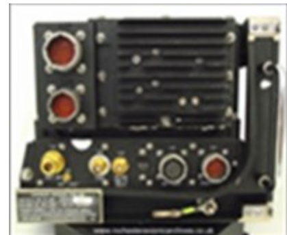
This is a Sonobuoy Receiver for the AQS903 system fitted to the EH101 Merlin.
