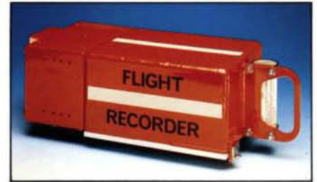
D51506 crash protected Cockpit Voice and Flight Data Recorder (CVFDR).
