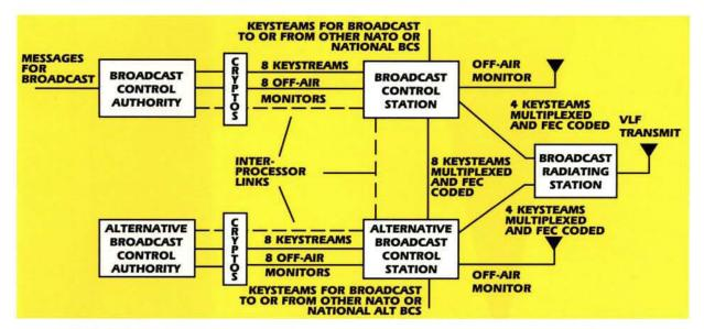
Radically improving the communications management and control of submarine forces, the GEC-Marconi Very Low Frequency (VLF) Control system has been designed to exploit the most recent technology and software developments.
