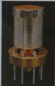
1. Opened-up view of the START Gyro.
