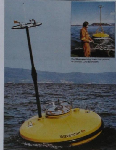
START is included in a Norwegian Seatex Wavescan Databuoy used for investigations into ocean wave motion.
