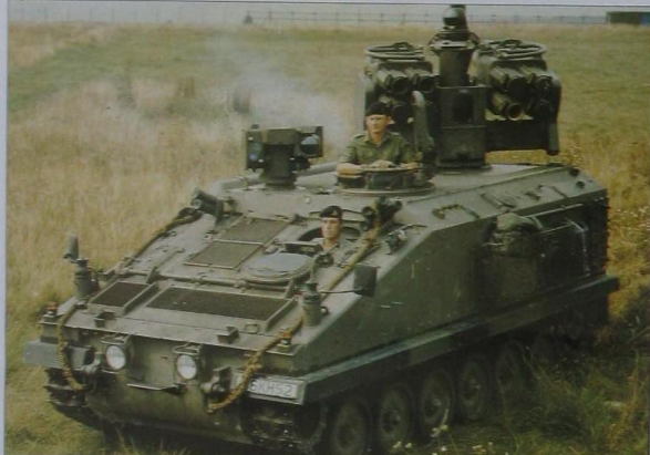
Thorn-EMI have selected START for measuring movement in all 3 axes of an elevated mast (seen here retracted) on an armoured vehicle. This is part of the British Army Air Defence Alerting Device which uses thermal imaging to detect air attack. 400 units have been ordered for this project, with options for a further 360. (Picture courtesy of Thorn-EMI).
