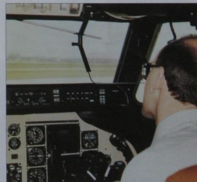
Steve Driver of ADD in the cockpit of a Gulfstream G2 during trials of a prototype, looking through the retractable combiner glass in its lowered position.
