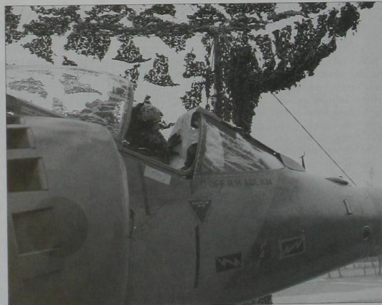
This Harrier GR5 cockpit is rather cluttered with the pilot's paperwork. The AMPA and colour map unit will dispense with the need for such techniques.
