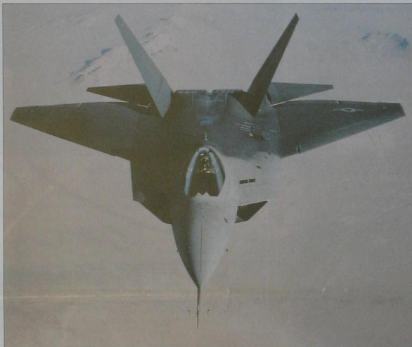
The 'stealthy' radar-resistant aerodynamic form is clearly shown in this view of the F-22 prototype.
