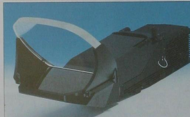
ADD's HUD represents the state of the art in wide angle HUDs and uses advanced holographic technology, similar to that also being developed for EFA.
