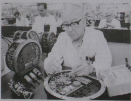
Below: Assembly of Control Sensors Units. In the foreground is Doug Fenning, Instrument Technician, subjecting a CSU to final checks prior to test, calibration, and delivery to customer.
