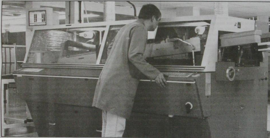
A nitrogen purged soldering facility used at Broad Oak on high volume commercial production to flow solder printed circuit boards. This machine eliminates the cleaning stage (no flux is used) and improves the quality of solder joints. The use of CFCs and other contaminants is also eliminated.
