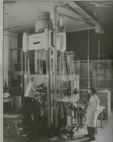
NNC engineers (above) have achieved a world first by successfully drilling and piercing under liquid sodium as part of the decommissioning project.
