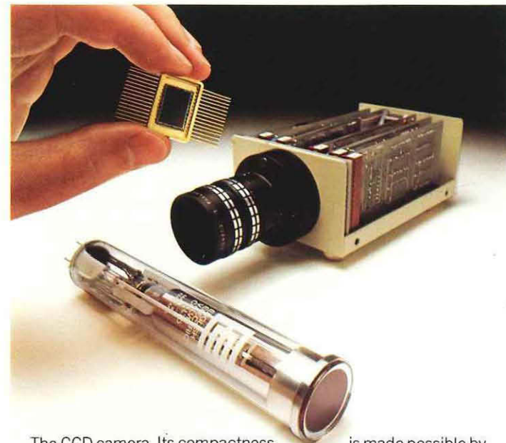
The CCD camera. Its compactness is made possible by the use of the semiconductor device (held above it) instead of an electronic tube (in the foreground).
