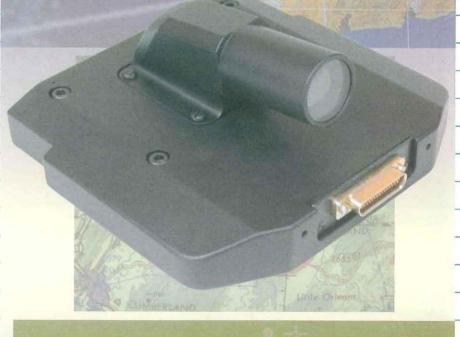
The only camera specifically designed as an integral part of the GEC-Marconi Avionics F-16 C/D Head Up Display, this high performance military camera provides a color image of the pilot's forward view to allow recording for mission debriefing, aircrew training and weapon analysis.
