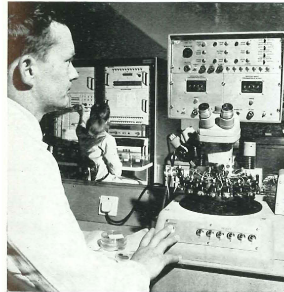
Production: a high-speed, computer-controlled, automatic testing system for microcircuits.
