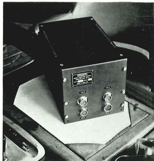
Microminiature Computers: the miniature 920M is a version of the '900' Series computer manufactured from microminiature integrated circuits. First applications are for defence purposes and space research.
