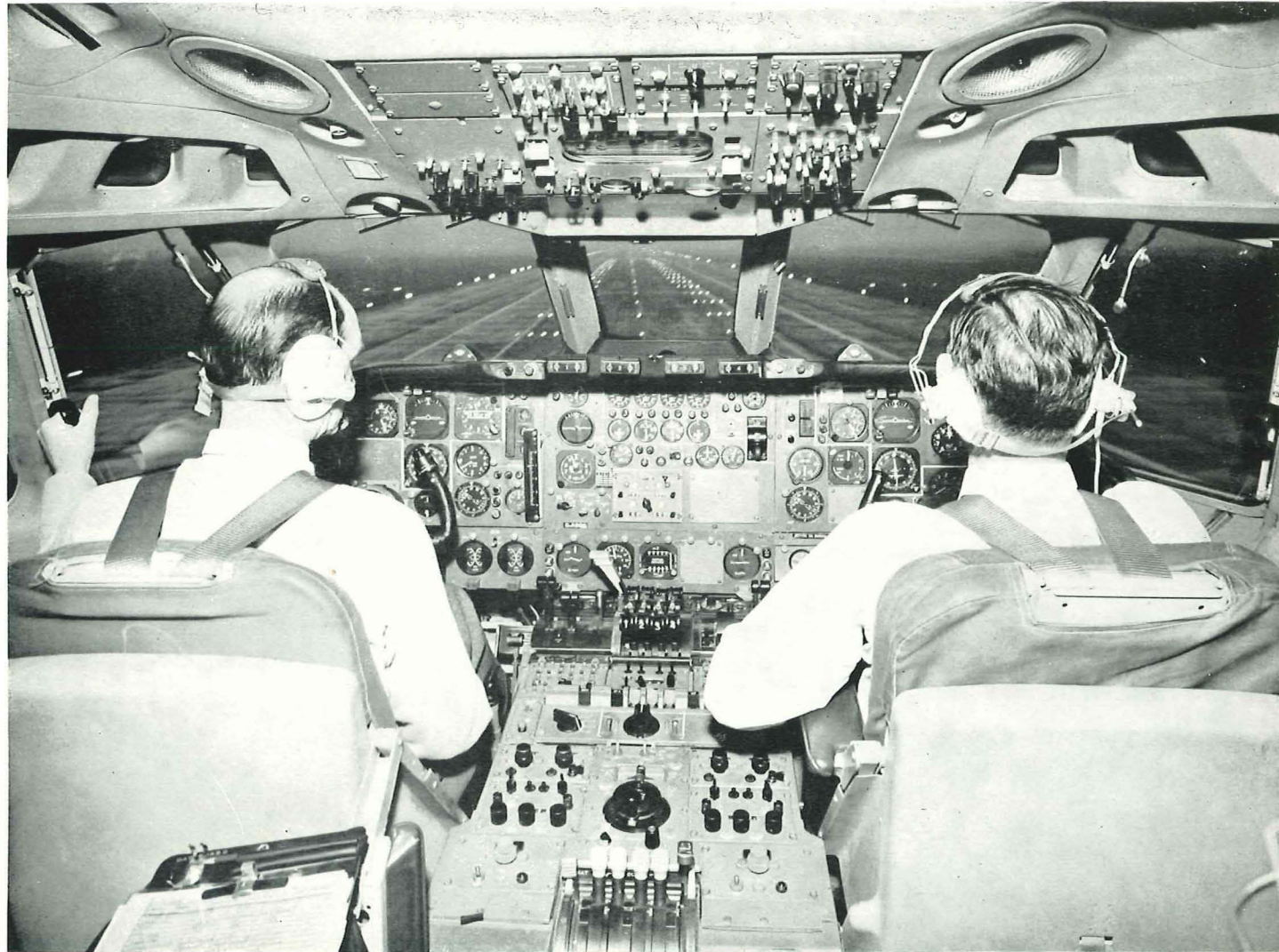
Blind Landing: VC10 flight deck during an automatic landing. Elliott failure-surviving automatic flight control and automatic landing systems are fitted in VC10 and BAC 111 airliners and have been specified for the Concorde supersonic jet airliner.
