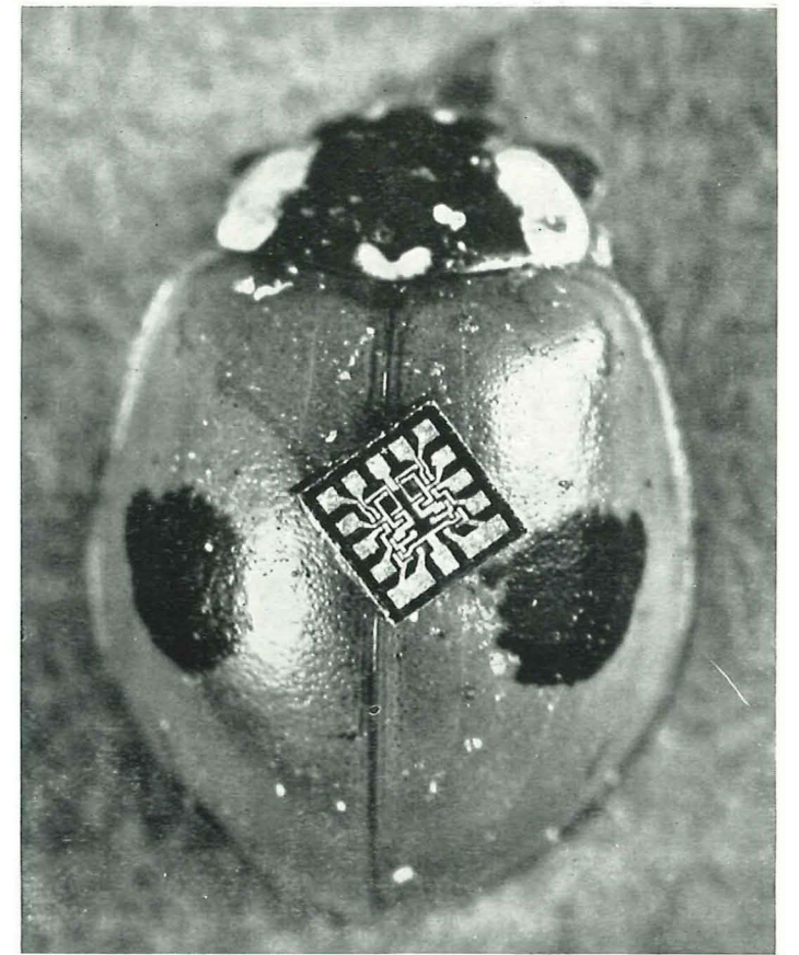
Microcircuits: a microminiature integrated circuit on the back of a hibernating ladybird. This type of circuit is mass produced at the Glenrothes microelectronics factory.
