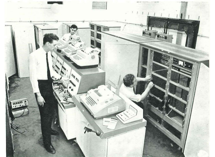
Process Control: commissioning-on-site an ARCH 2000 computer direct digital control of a large process plant.
