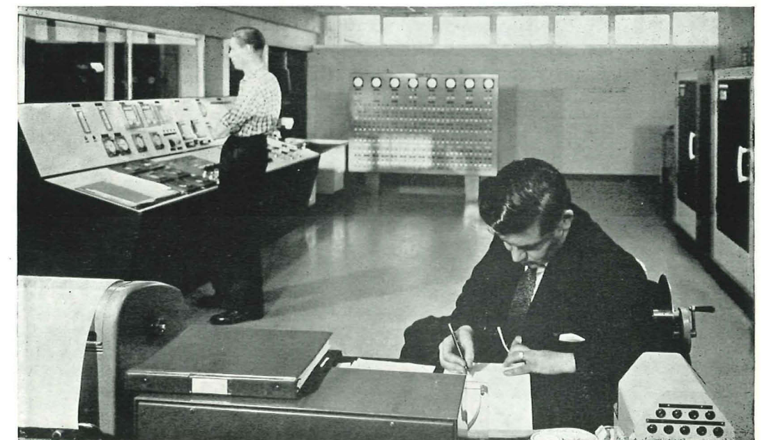
The electronic digital computer is the most important single element in all true automation systems. This Elliott 'on-line' computing system, which controls a paper making machine, has increased throughput by 15%.
