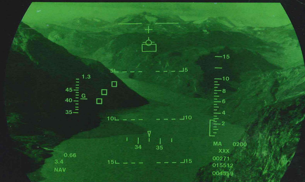
1 to 1 FLIR Imagery with Flight Symbology and Target Cueing
