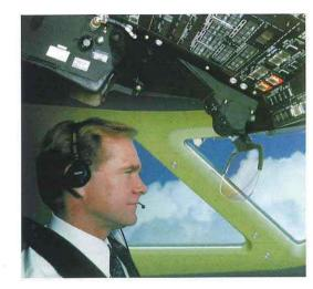
The primary advantage of a HUD is the ability to present important aircraft performance and control information to the pilot in his forward field of view. Without reference to head-down instruments, the pilot is continually aware of the aircraft's position, true flight path and energy state.
