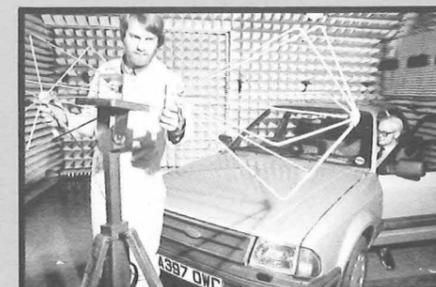
Setting up a vehicle for EMC testing to demonstrate its ability to withstand high RF fields
