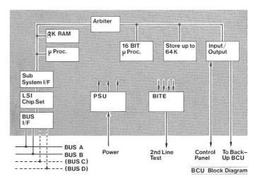
The BCU contains plug in modules, using large scale integrated components for economy and reliability. The BCU is housed in a 1/2 or 3/4 ATR short rack-mounted unit, the size depending on the module options chosen by the customer. These are decided by the complexity of the system and the comprehensiveness of control demanded.
