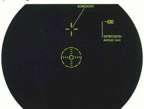
**Electronically Depressible Reticle** For simple applications when no avionics inputs are available.
