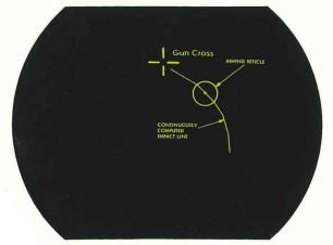
**Continuously Computed Impact Line** Visually portrays the path bullets will take by using a tracer line passing through an aiming point. An easy-to-use, accurate air-to-air solution.
