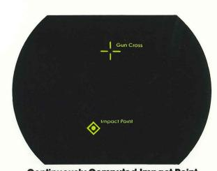
**Continuously Computed Impact Point** Uses aircraft flight data to predict the impact point of bullets and rockets on the ground.
