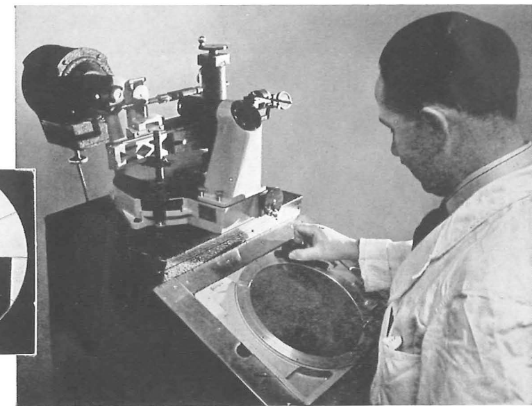
The Projector. A magnified silhouette is thrown on a glass screen.
