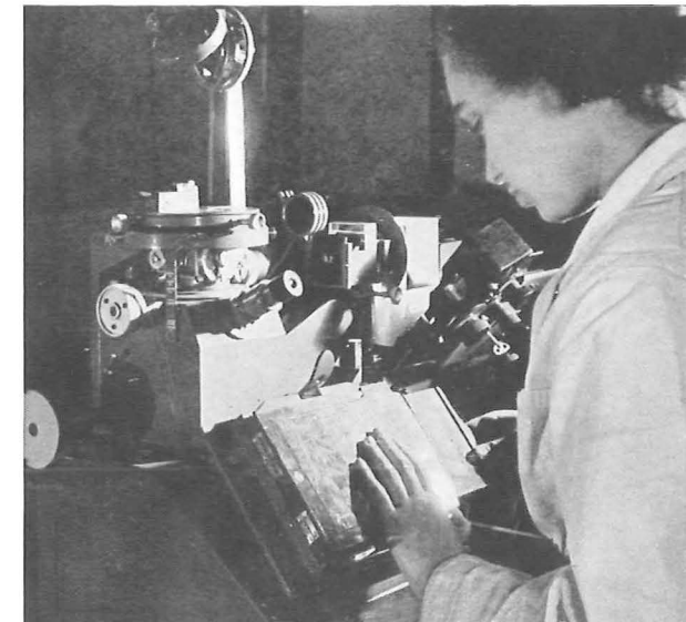
Photographing a Micro-structure. Metallurgy plays a vital part.
