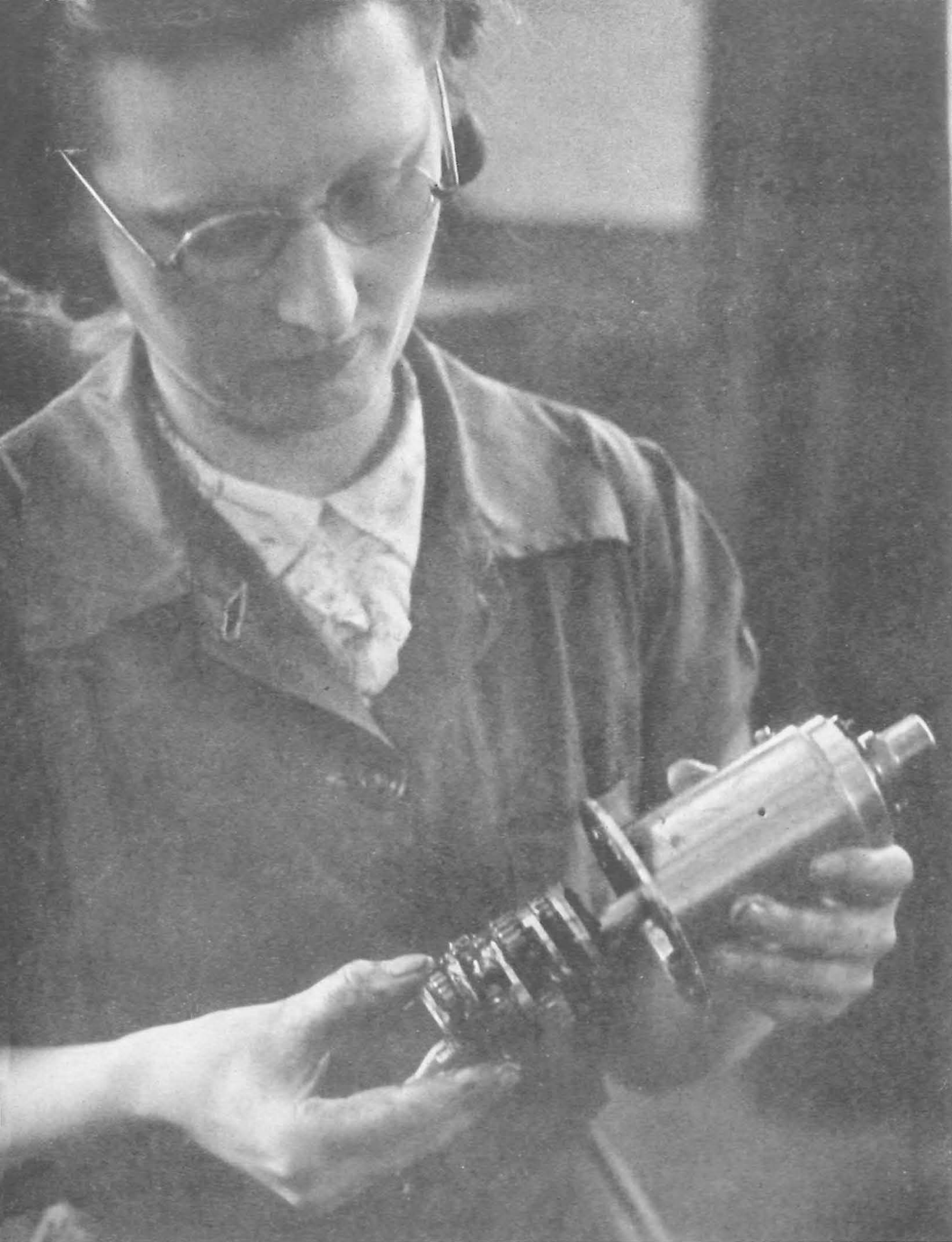
Component tests complete. The gear unit is heavily greased, for many years of trouble-free wear, and assembled.
