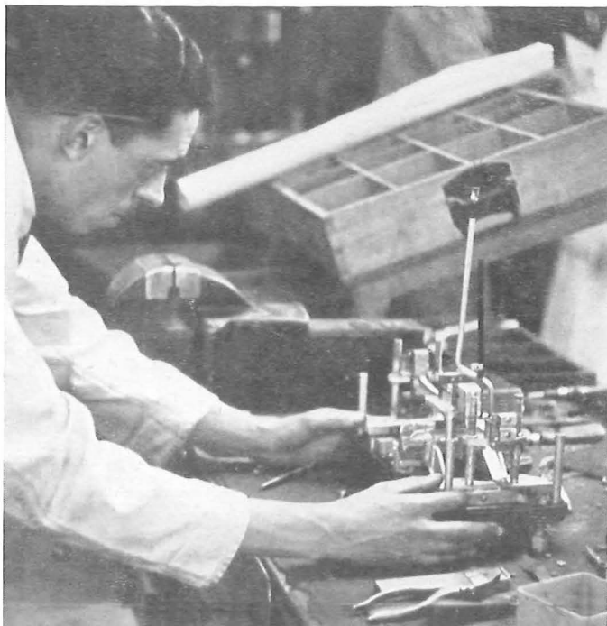
The birth of a Weighing Machine. Mechanism being assembled.
