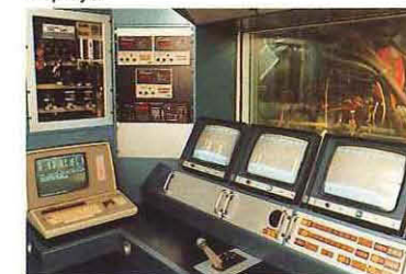
Automated powerplant test system, bought by four air forces, to save fuel and manpower and prolong engine life.
