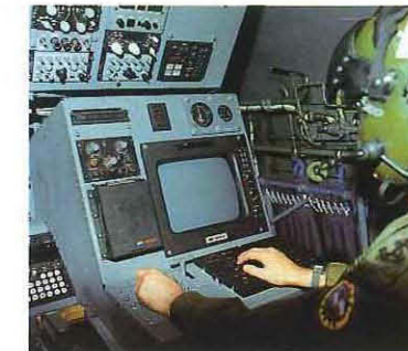
One of the Queen's Awards winning AQS-900 series of acoustic systems, processes and displays both sonobuoy and dipping sonar data.
