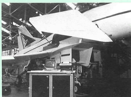
1553B Integration Facility with EAP at BAe Warton.
