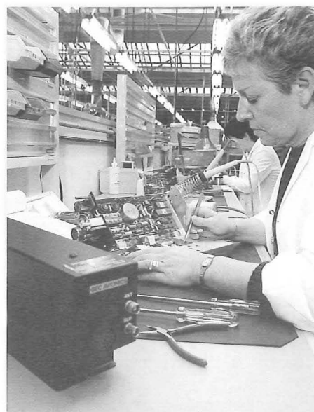
Tactical Air Navigation systems (TACAN) being assembled for the Shorts Tucano trainer aircraft
