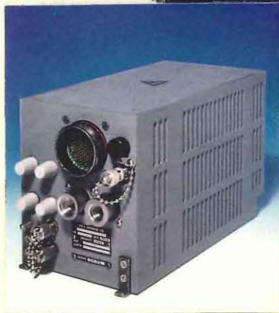
Miniature Standard Central Air Data Computer (MSCADC)
