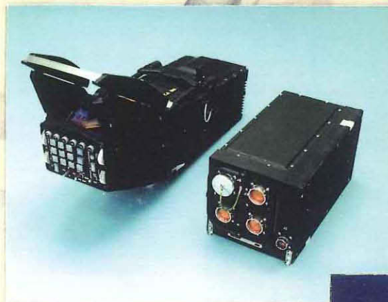
F-16 Head Up Display and electronic control unit
