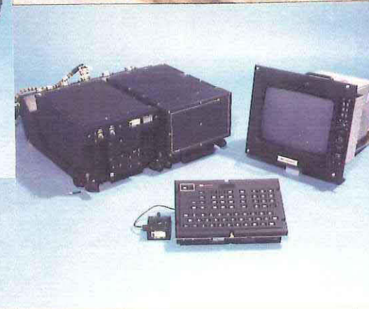
AQS 920 Acoustic Processing System Hardware
