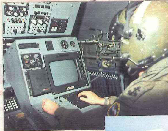
Acoustic Processing System for the RN Sea King Mk 6
