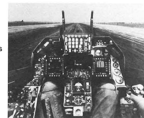
USAF front pilot's view through the new wide angle HUD for the General Dynamics F-16 C/D fighter.
