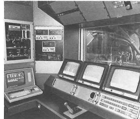
Automatic Powerplant Test installation at RAF Honington for Tornado's RB199 engines.
