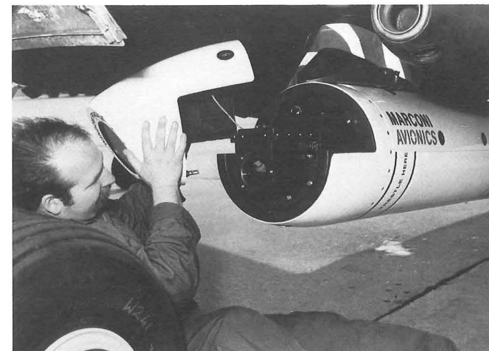
This FLIR (forward-looking infra-red) pod, fitted on a combat aircraft, is made entirely from Thermal Imaging Common Modules.
