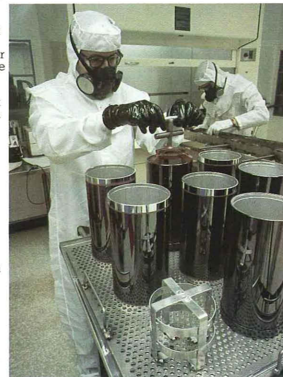
A B Dick of Chicago, USA is one of few companies in the world which manufactures selenium drums for use in most xerographic copying machines. The company produces drums for copier manufacturers in several countries.
