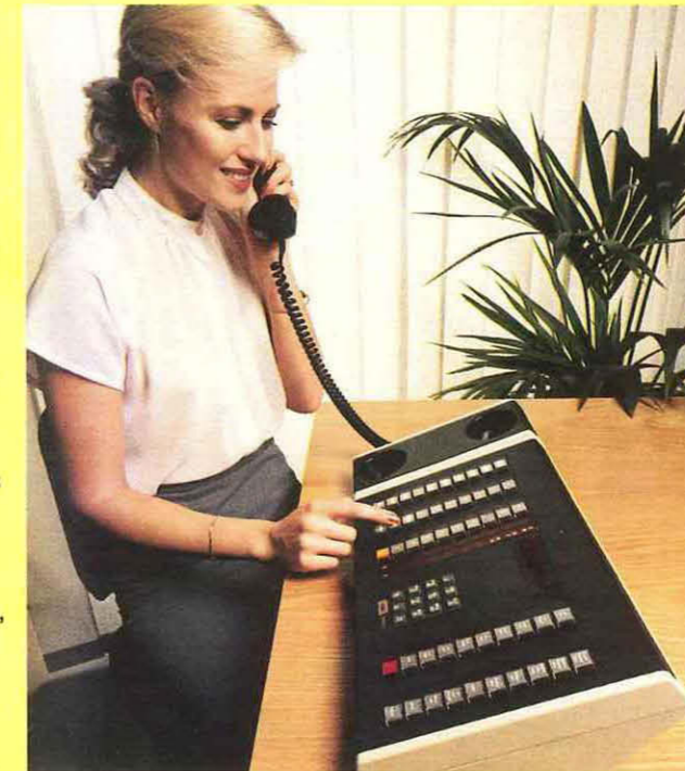
Reliance Systems Ltd, Wellingborough is having much success with its popular SL-1 private automatic telephone exchange. Some of Britain's major companies have installed or ordered the exchange which caters for up to 5000 extensions. The picture shows the SL-1 switchboard.
