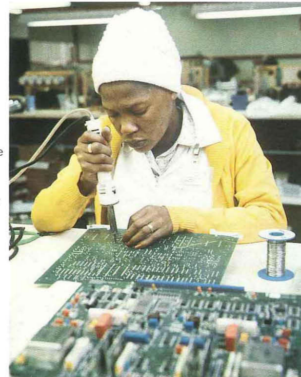
If a computer detects a fault in a printed circuit board at a new factory of GEC South Africa (Pty) Ltd at Kew, Johannesburg, a skilled operator makes a correction. Meticulous attention is given to on-the-job training for all employees.
