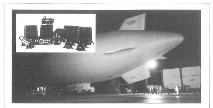
It is interesting to note that the equipment is now over five years old and has been operated for many hours in laboratory and hangar environments as well as actual flight hours. During this time there has been no significant degradation in performance of the active optical components. Any problems which have occured within the optical system have been in the fibre optic connectors.
