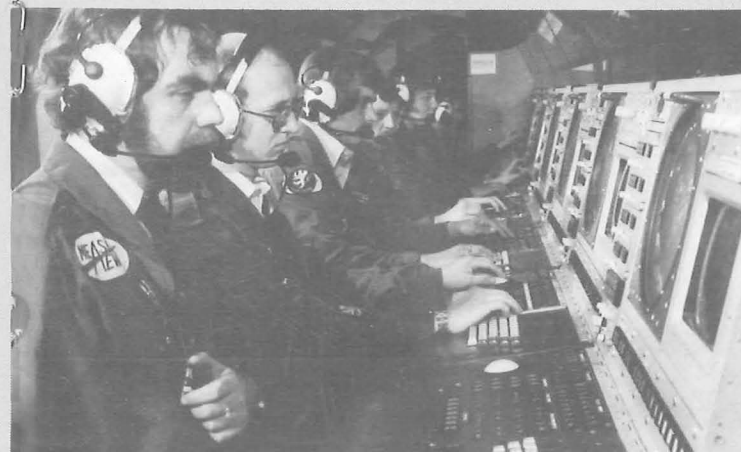
Above The mission system avionics rig at Marconi Avionics' Radlett plant is complete with fore and aft scanners. The forward aerial is raised relative to its position in the aircraft. Left AEW operators at their positions in the rig
