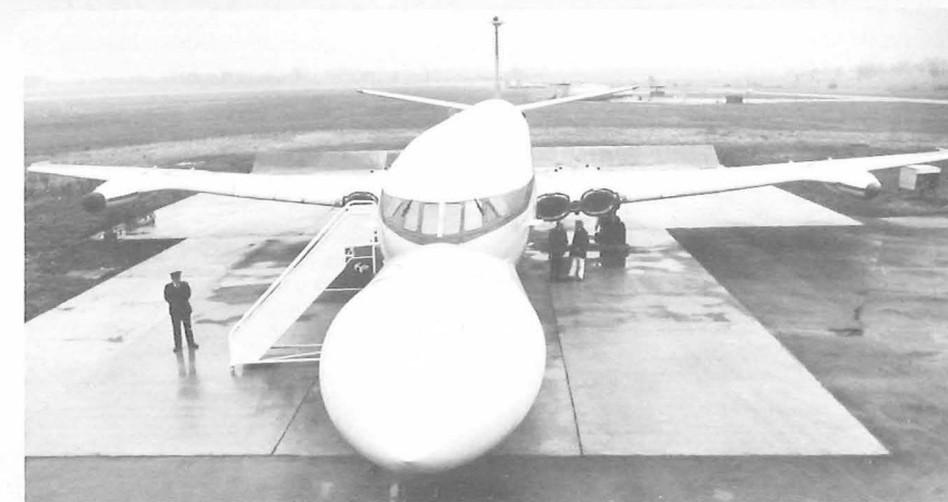
Heading The first British Aerospace Nimrod AEW.3 airborne early warning aircraft displays its pneumatic lines, first hinted at below when the Comet radar trials aircraft was unveiled
