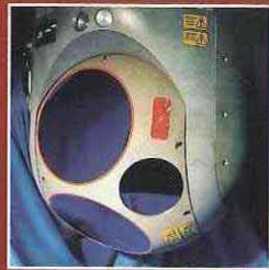
Infrared counter-measures turret
