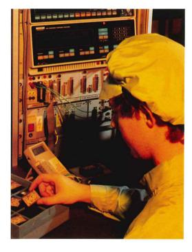
Utilising Thick Film printing and firing techniques, electrical conductor and resistor patterns are produced on a ceramic substrate base. To this base, active components from individual diodes and transistors to Custom VLSI integrated circuits are incorporated. The functional substrate is then packaged to meet customer, military and aerospace specifications.
