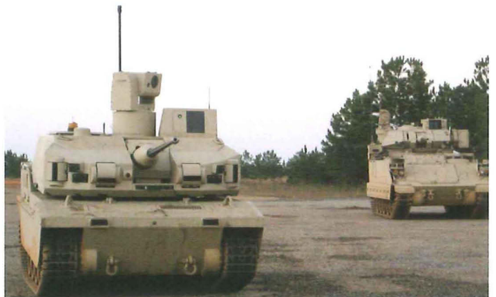
The Black Knight Unmanned Combat Vehicle (left) is wirelessly tele-operated from within the Bradley Technical Demonstrator (TD) and acts as a scout or wingman to the Bradley TD.
