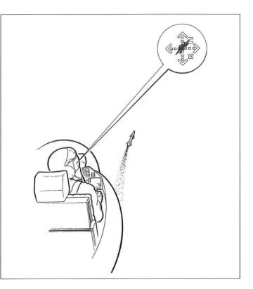
The Alpha Sight system comprises an optical sub-system, a mount assembly and associated electronics. Sighting and cueing information is presented to the pilot by means of the high brightness LED reticle relayed by a prism and reflected into the pilot's eye via a dichroic patch coated on the inner surface of the clear visor. All the equipment subassemblies fit into a standard Alpha helmet, with minimum change to the basic helmet structure.
