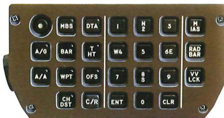
Up Front Control Panel
