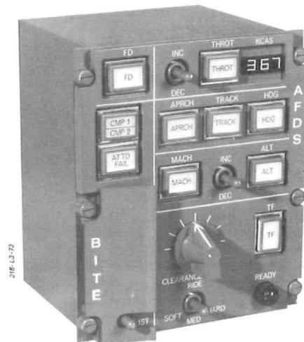
Figure 13 Pilot's control panel
