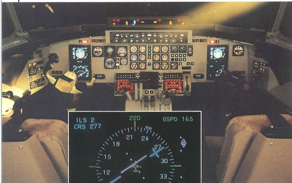
Civil EIS installation for the ATP
