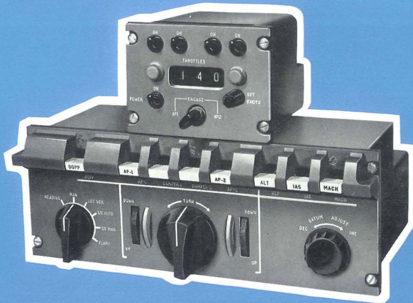
FIG. 5—AUTOPILOT DUAL CONTROLLER AND AUTOTHROTTLE DUAL CONTROLLER
