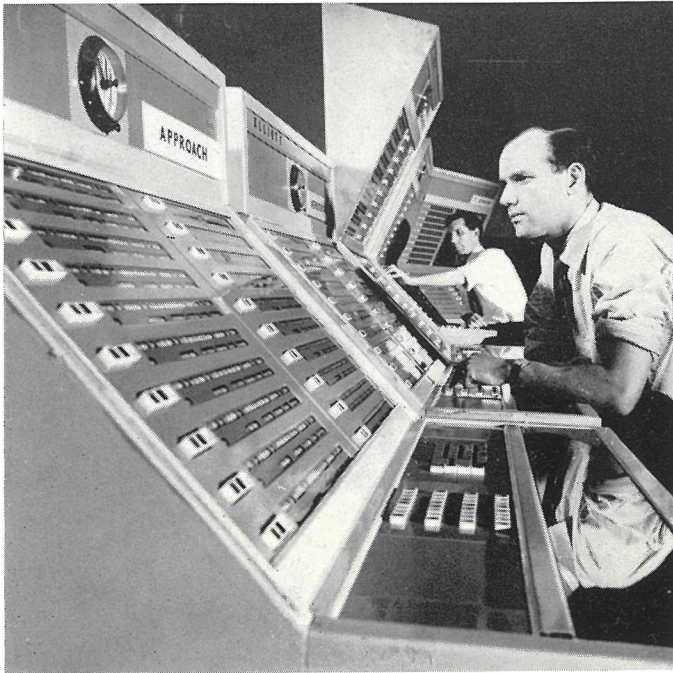
Euclid digital air traffic research simulator
