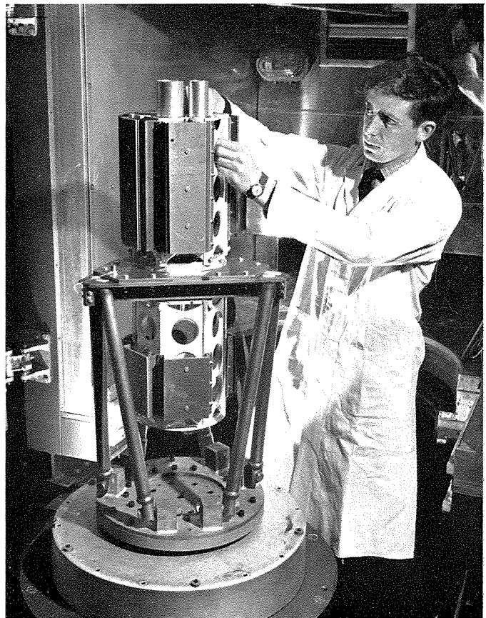
Telescope structure for passenger experiment in OAO-C satellite
