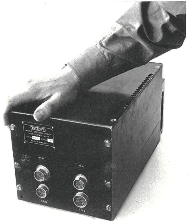
MCS 920M microminiature computer for digital inertial guidance of Europa launch vehicles (left)
