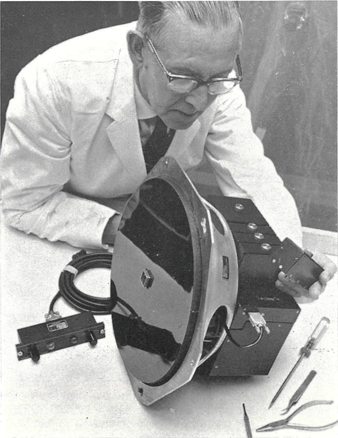
The Visor terrain-warning radar for airliners
