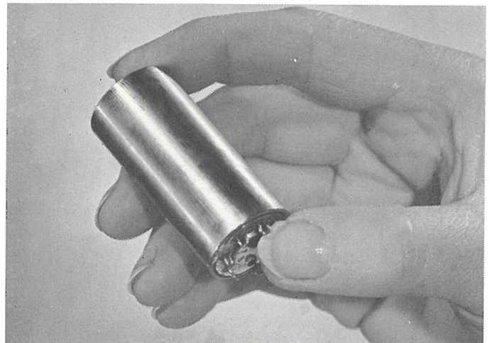
Sub-miniature, precision rate gyro
