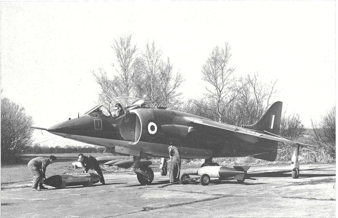
Hawker Siddeley P.1127 V/STOL close-support aircraft
