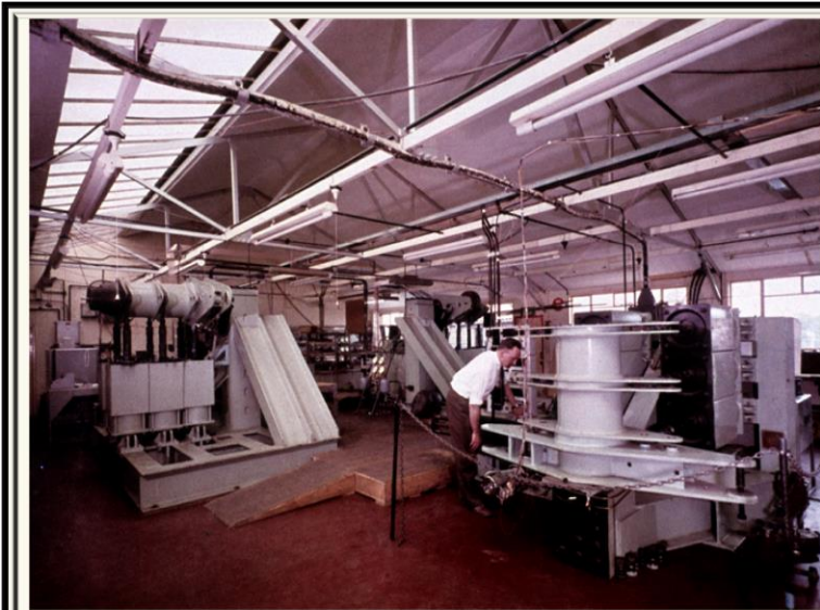
The Test Rig for the TSR2 Flight Control System. This was located in in one of the Huts at Rochester in about 1965.
