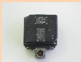
This Gyro was photographed at the Leicester National Space Centre where the description cites its use in the WWII German V2 Rocket Guidance system.
