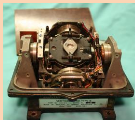
This Gyro was photographed at the Leicester National Space Centre where the description cites its use in the WWII German V2 Rocket Guidance system.
