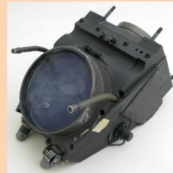
The A-7 Corsair II Head Up Display optics showing the large exit lens.
