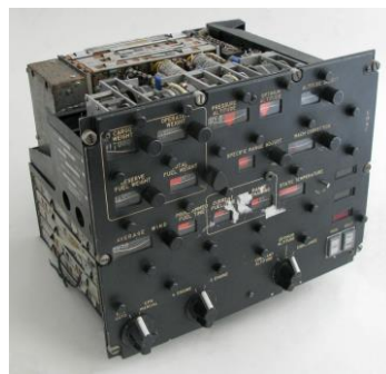
The C-5A Energy Management Computer is shown above and the Crosswind Casting Computer to the right
