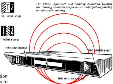
The Elliott Approach and Landing Situation Display is a head-up display which presents to the pilot simple and unambiguous information of autopilot state and the aircraft's position relative to the flight path. The display is associated one with each left and right monitored autopilot, radio altimeter and radio systems, and is designed for mounting on the top surface of the glare shield, one in front of each pilot, such that it does not interfere with the pilot's normal field of view.
