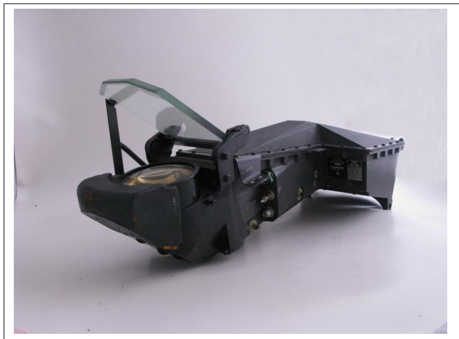
The Strike Sight PDU for the Royal Navy Buccaneer. This early HUD has the large valve high voltage power supply in the box at the forward end.
