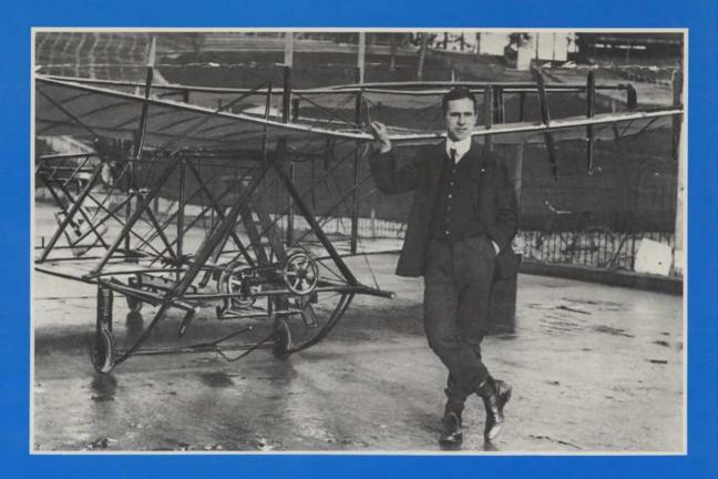
Above (Syndication International): Soon after A.V. Roe arrived at Brooklands in 1907 he posed for this picture with what he described as the first man-lifting machine built in England which left the ground. The specifications of the Roe Biplane were: length 23 feet wingspan 30 feet weight 350 lb. power 9 h.p. JAP (later fitted with 24 h.p. Antoinette) speed 38 m.p.h.
