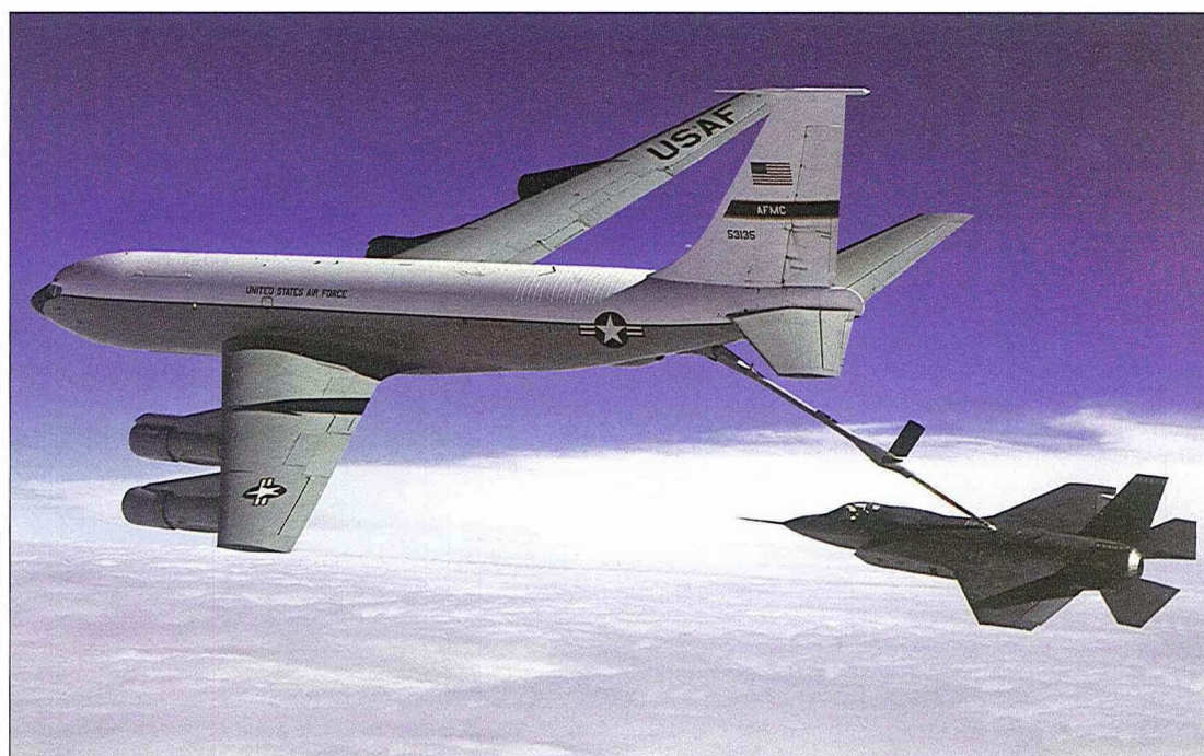
A magnificent air-to-air shot of the X-35 advanced tactical fighter during flight refuelling trials with a KC-135 tanker aircraft. Two versions of the X-35 were proposed, one V/STOL and one conventional.
