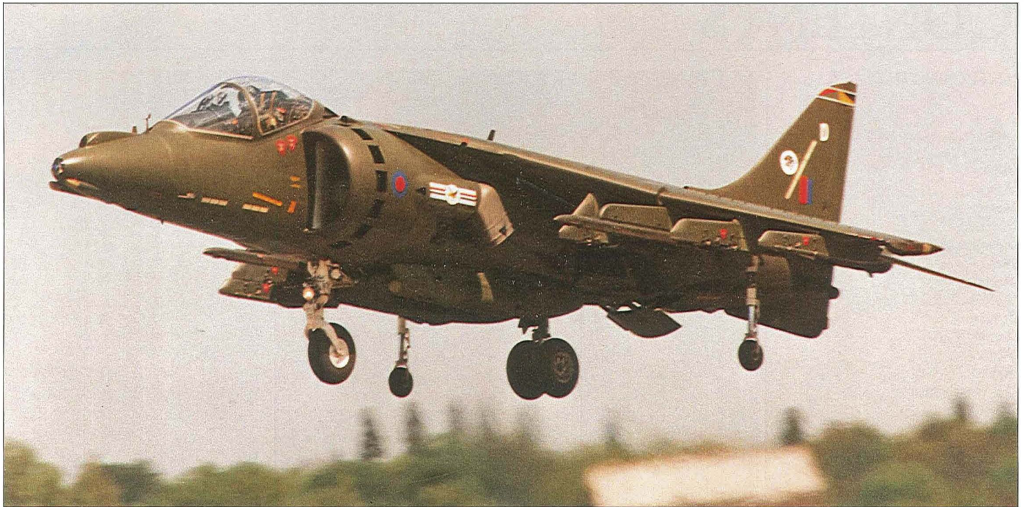
A Harrier GR.7, the RAF's equivalent of the US Marine Corps' AV-8B, pictured at the point of transition from vertical to horizontal flight.
