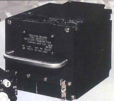
Transmitter / receiver type AA35001-2 ARINC 429 control
